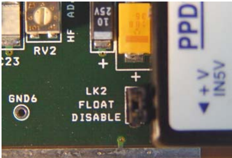
Figure 2-1. Float Enable/Disable Jumper
